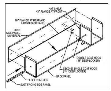
**Step 3:** Attach the second side panel and the right rear leg to the assembly of Step 2. On 15" deep lockers attach a third single coat hook. On 18" deep lockers substitute a single coat hook with a double bend for the third single coat hook and install the coat rod as shown on page 3. The locker chassis is now complete.
