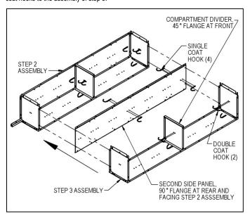
**Step 5:** Attach the third top shelf, the third bottom shelf, and an additional two coat hooks to the third back panel as in steps 1 and 3.
