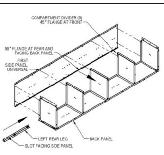
**Step 3:** Attach the second side panel and the right rear leg to the assembly of Step 2. The locker chassis is now complete.
