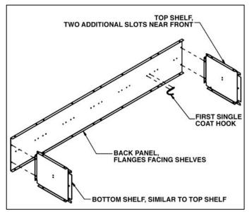
**Step 2:** Turn the back panel on its back with the shelves pointing upward. Attach the first side panel, the left rear leg, and the first hat shelf to the assembly of Step 1. Attach a single coat hook with a double bend, this will accommodate the coat rod).
