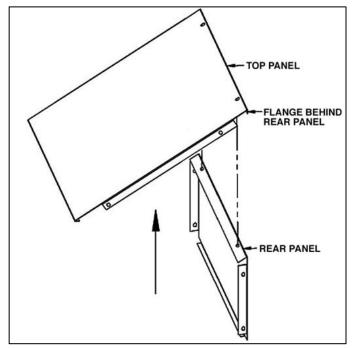
Step 2: Assemble the side panels to the top panel and rear panel with  $#10 - 24 \times 3/8"$  long slot less screws and #10 nuts (provided).
