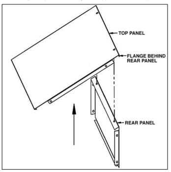
**Step 2:** Assemble the side panels to the top panel and rear panel with #10 -  $24 \times 3/8$ " long slot less screws and #10 nuts (provided).
