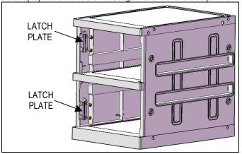
**Step 11.** Install screws and hole covers where side panels join to top panels and base panel. There are 22 screws and hole covers on each of the two sides of the assembly (44 in total).
