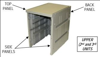
**Step 6.** If no optional sloping hood is ordered, install the three (3) filler strips into the recesses in the top panel of the upper unit.
