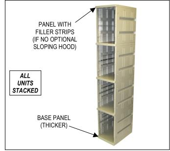
**Step 8.** Insert one (1) of four (4) divider panels in between each of the horizontal panels previously installed. The panels slide in grooves in the side panels and may need the use of a soft rubber mallet to fully engage the two small latch pins into the holes in the front edge of the side panels.
