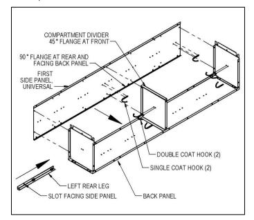
Step 3: Attach the second top shelf, the second bottom shelf, and an additional two single coat hooks to the second back panel as in step 1.
