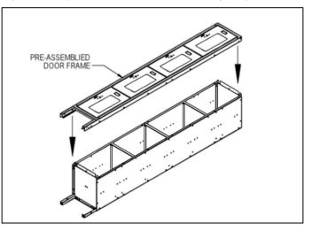
**Step 5:** Tighten all fasteners checking for squareness of the locker while tightening. Attach optional sloping hood, end bases or front base (see pages 4 and 5).
