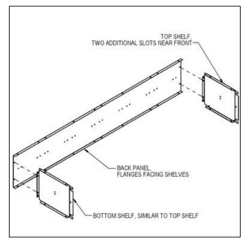
**Step 2:** Turn the back panel on its back with the shelves pointing upward. Attach the first side panel, the left rear leg, and five compartment dividers to the assembly from Step 1.
