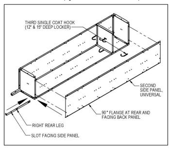
Step 4: Attach the pre-assembled door frame onto the assembly of Step 3.
